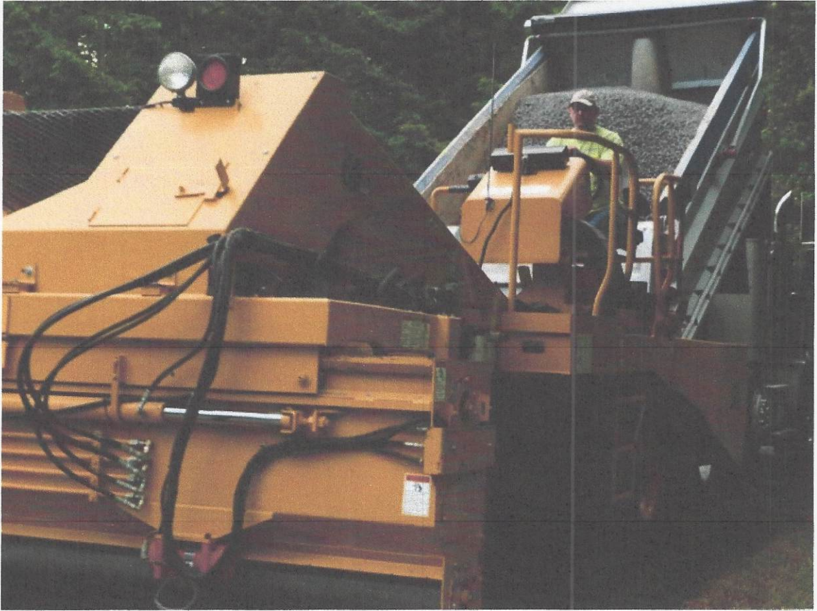
Computer controlled gravel spreader that is attached to a dump truck.
